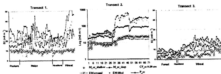
Figure 1.  $EC_a$  values measured with EMRC-120 lifted (0-1.0 m), EMRC-120 ground (0-1.5 m), Martek\_shallow ( $M_{ec}$  0-0.20 m), Martek\_deep ( $M_{ec}$  0-0.45 m), Conductivity fork ( $CF_{ec}$  0-0.25 m) and Percometer ( $P_{ec}$  0.20 m) in 3 transects
