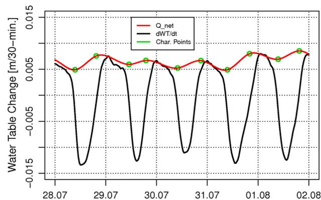
**Fig. 3** Graphic representation of the empirical  $ET_{gw}$  estimation method according to Gribovszki et al. (2014).  $Q_{net}$  is replenishment rate, and  $dWT/dt$  is the time rate of change in GWL, Char. Points are the characteristic points of the replenishment rate
